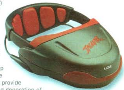
This prototype Jaguar HMD lacks the unusual infra-red tracking 'bug eyes' of the final unit
